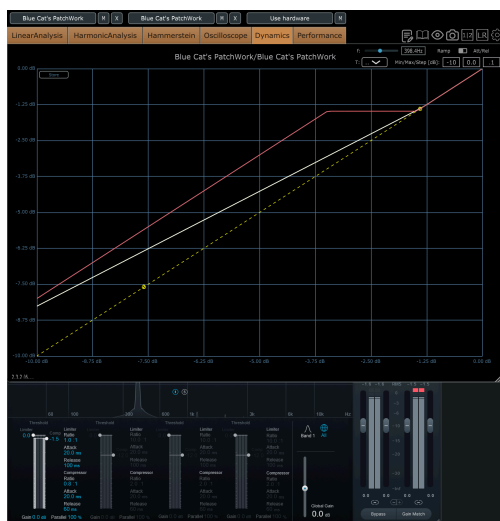
Ranged upward compression (red) versus non-ranged upward compression in Ozone Dynamics (white)
